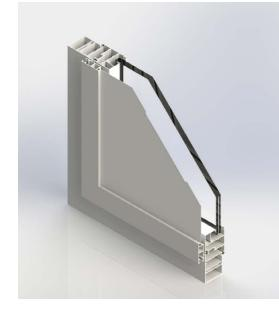
TWF.ACA.50.OS is a 50mm casement window with a restricted opening of 8 inches, majorly used in places where only basic ventilation is required such as washrooms, store areas etc. The handle, in this system is integrated in the frame, which allows the magnetic fly screen to stay permanently on the opening.
