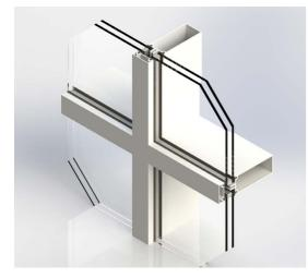
TWF.ACW.4565 is designed keeping in mind to achieve larger double height spans with avoiding the structural horzital member. The depth of 108mm gives freedom to go upto 7000mm wihtout any horizonatal strutural member resulting in a very sleek Elevational look.
