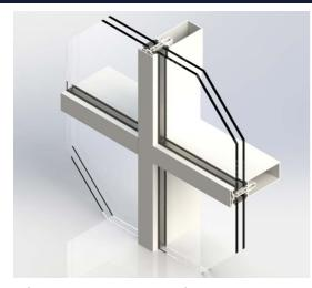
With a mere 40mm face width and thermal break insulation, TWF.ACW.4090 gives a very sleek and slim look without compromising on strength and durability. The unique feature in this system is that we can provide all kinds of different thicknesses in glasses as it has an adjustable notch. The system has outstanding performance and its ease of installation makes it possible to suit individual project requirements.
